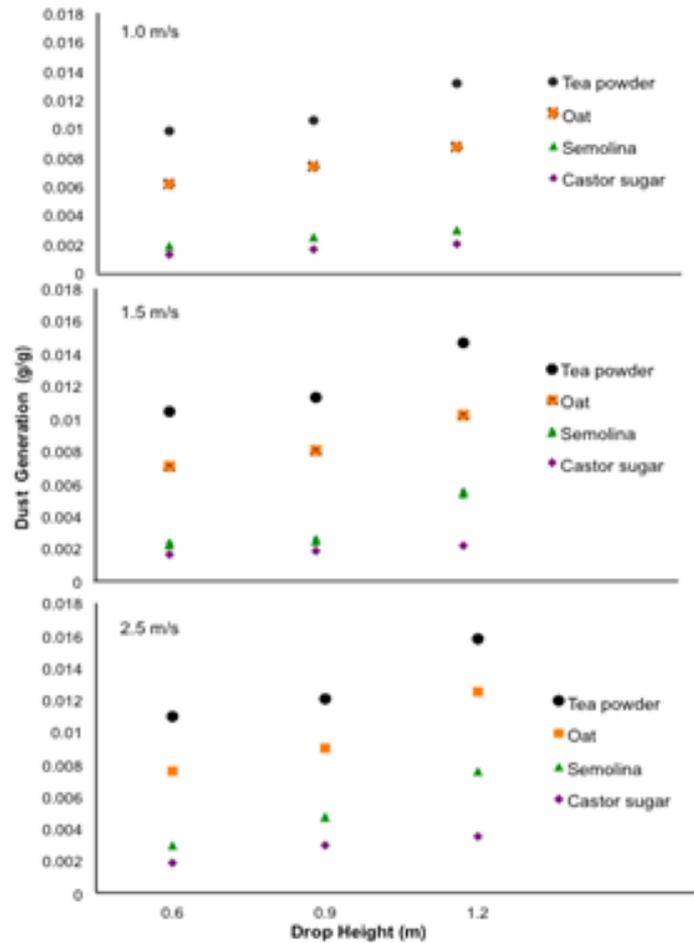
Figure 3. Influence of drop heights and conveying velocities on airborne dust generation
