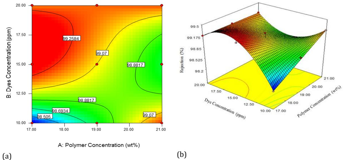
Figure 1: (a) 2D contour and (b) 3D Plot showing interactive effects of varying dye concentration and polymer concentration values on percent dye rejection efficiencies for SDS surfactant
