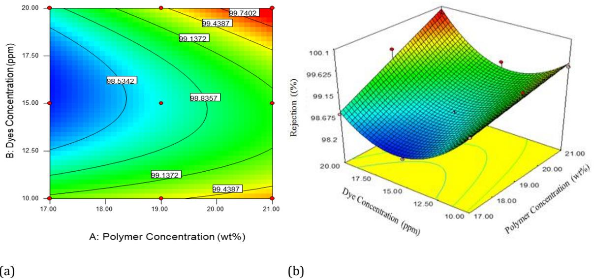
Figure 2: (a) 2D contour and (b) 3D Plot showing interactive effects of varying dye concentration and polymer concentration values on percent dye rejection efficiencies for CTAB surfactant
